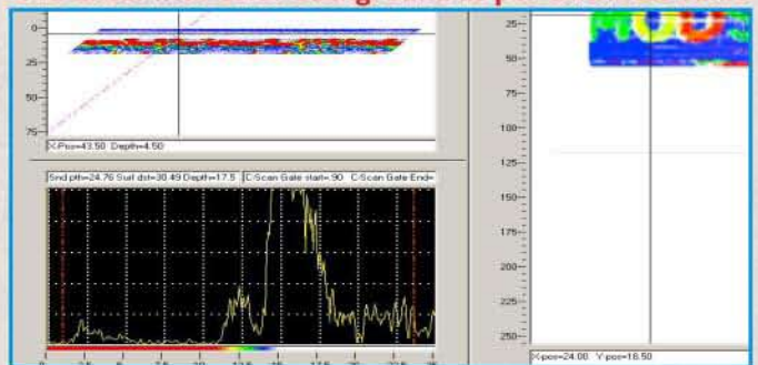
C-Scan can be generated for 'selectable' thickness range.
