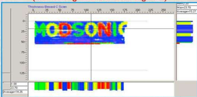
C-Scan ,Side view and bottom view can be seen with thickness based color coding
